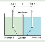
values, this layer will have a low hydrogen concentration. However, at low pH values a large number of H+ ions diffuse in the layer. By measuring the generated electrical potential (E) in the layer the corresponding pH can be computed.
